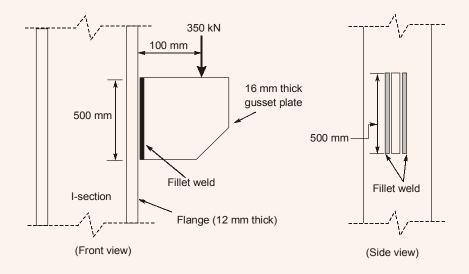
The maximum resultant stress (in MPa, round off to 1 decimal place) on the fillet weld along the vertical plane would be\_\_\_\_\_.
