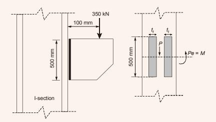
$$P = 150 \text{ kN}, e = 100 \text{ mm}$$
