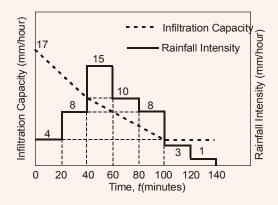
The infiltration capacity at the start of this event (t = 0) is 17 mm/hour, which linearly decreases to 10 mm/hour after 40 minutes duration. As the event progresses, the infiltration rate further drops down linearly to attain a value of 4 mm/hour at t = 100 minutes and remains constant thereafter till the end of the storm event. The value of the infiltration
