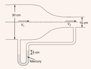
When the water flows, the differential manometer shows a deflection of 8 cm of mercury (Hg). The values of specific gravity of mercury and water are 13.6 and 1.0, respectively. Consider the acceleration due to gravity, g = 9.81 m/s<sup>2</sup>. Assuming frictionless flow, the flow rate (in m³/s, round off to 3 decimal places) through the duct is \_\_\_
