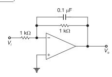
Solution: Output voltage of inverting amplifier
