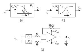
The cut-off frequencies of  $F_1$  and  $F_2$  are  $f_1$  and  $f_2$ , respectively. If  $f_1 < f_2$ , the resultant circuit exhibits the characteristics of a:
