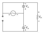
During negative half cycle of the supply under steady-state.
