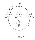
$$i = \frac{(100 \angle -120^{\circ}) - (100 \angle 120^{\circ})}{j1} + \frac{(100 \angle 0^{\circ}) - (100 \angle 120^{\circ})}{-j1}$$
