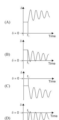
**Solution:** For alternator rotor angle is positive, after fault occurring this rotor angle increases.
