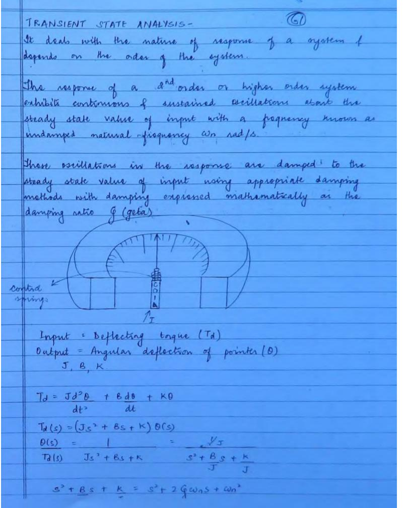
$con = \frac{|K|}{J}$  rad/sGia B. Undamped Natural progressing in rad/a - Damping Ratio & [Geta] 52 + 29 was + con2 Effect of Damping on Nature of Response  $\frac{C(s)}{R(s)} = \frac{\omega n^2}{s^2 + 2G\omega ns + \omega n^2}$ s3 + 2 goons + wn2 =0 = - 29 cons I J4g - wn - 4con - g wn I wn /g2-1  $D = G^{2} - 1 = 0 \Rightarrow G = 1$   $D = G^{2} - 1 < 0 \Rightarrow G < 1$ 0 = G' + 70 = G 71
