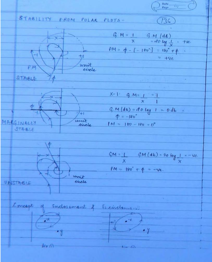
A point is said to be enclosed by a contour if it lies to the right side of the direction of the contour. A point is said to be encircled if the contour is a closed path. point & los is said to be enclosed whereas direction direction. In Polar plots if the critical point -1+jo is not enclosed then the system is said to be stable THEORY OF NYQUIST PLOTS Principle of Mapping S-plance P(D- plane P(3) = S+2 P(0) = 0+2 = 2 P(-j5) = -j5+2
