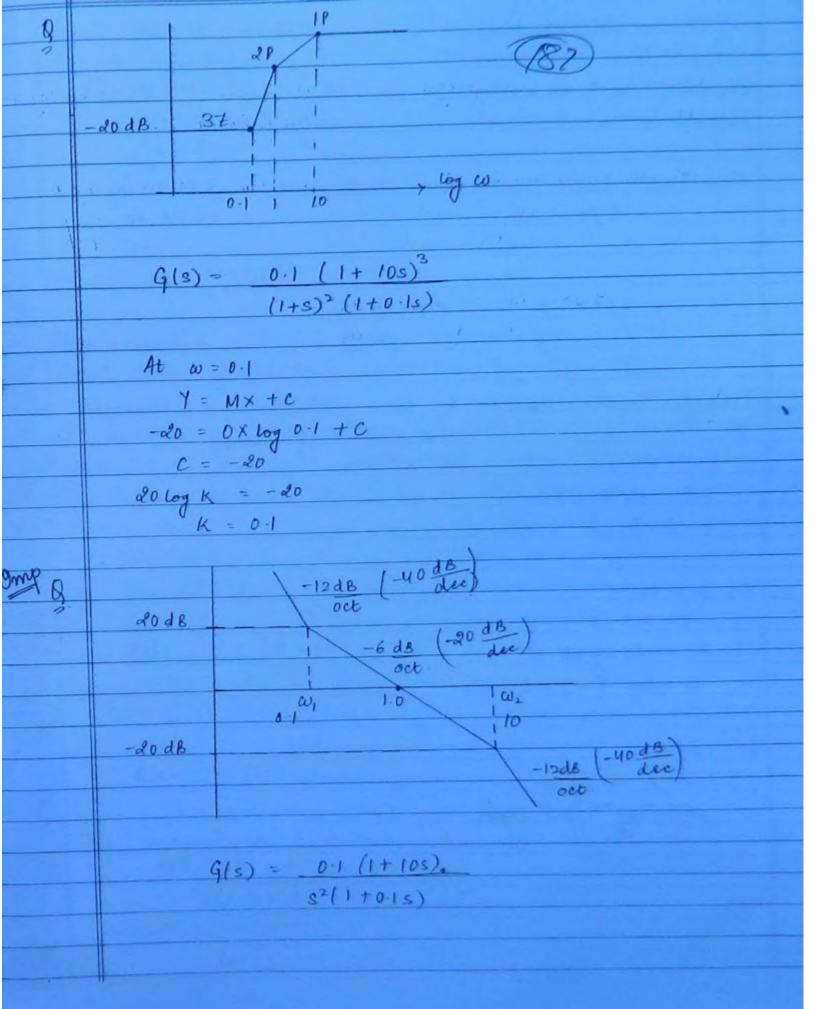
DECADE SCALE 188 OCTAVE SCALE  $\omega_2 = 2\omega_1$  $\omega_2 = 10 \, \omega_1$ dB value = I do x n log w dB value = 1 20 x n log w magnitude Magnitude Slope (m) = Idoxnlog2 Slope (m) = 1 do x n log 10 = 16 xn dB = 1 doxn d8 Idande & I doxndB oct dec' Second Line choise a line which james through At w=1 a known frequency. Y = MX +C 0 = -20 log 1 + C At w= w, Y = MX + C 20 = -20 log w, +0 W1 = tog (-1) = 0.1 1/s At w= Wz -do = -do log w = + 0 W2 = log (1) = lon/s
