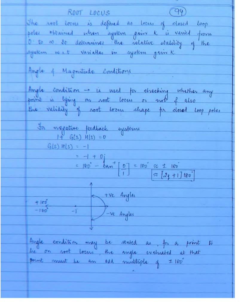
Magnitude condition is used for finding the magnitude of system gain k at any point on the root locus
